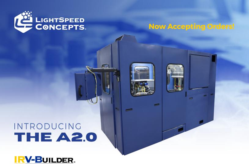
3D sand mold and core building is now affordable & economical, faster, and greener, enabling leaner processes and lighter castings. The IRV-Builder® is sand agnostic, utilizes BlueNano® binder, infrared, and single pass building for maximum efficiency. No post processing in microwaves or ovens is required.
